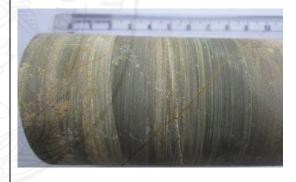
Fig.10.10. Core sample of glauconitic shale, borehole RKS-5, Jhiri Formation, near Gothra
