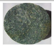
Fig.10.11. Core sample of glauconitic sandstone, Taragarh sandstone, borehole RKS-7, near Garain
