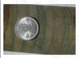
Fig.10.9. Core sample of glauconitic sandstone, borehole RKS-5, Jhiri Formation, near Gothra
